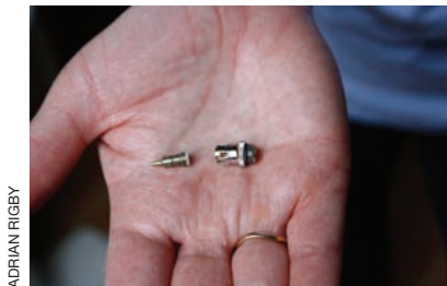
Nozzle taken apart for cleaning
