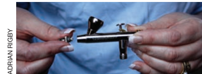
Removing or unscrewing the nozzle
