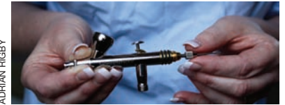
Removing the needle
