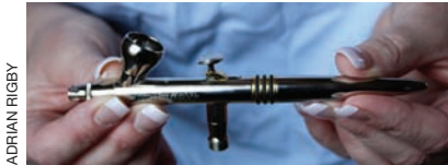
Unscrewing the main body to get to the needle
